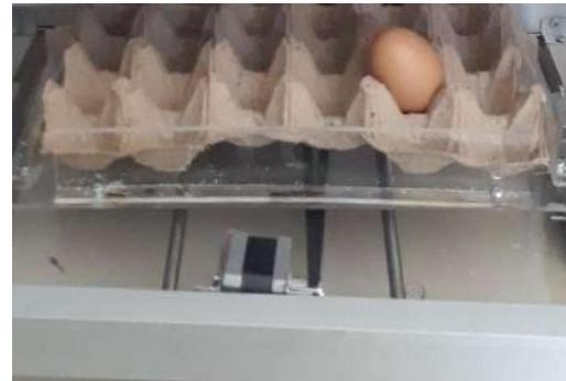
Gambar 9. Posisi Motor Stepper Axis X
