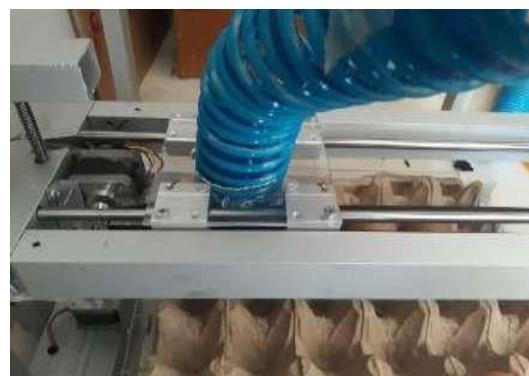
Gambar 10. Posisi Motor Stepper Axis Y
