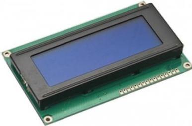
Gambar 2.5 LCD 20x4
